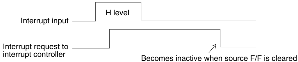
Figure 9.3-3 Interrupt Source and Interrupt Request to Interrupt Controller when Interrupts are Enabled
